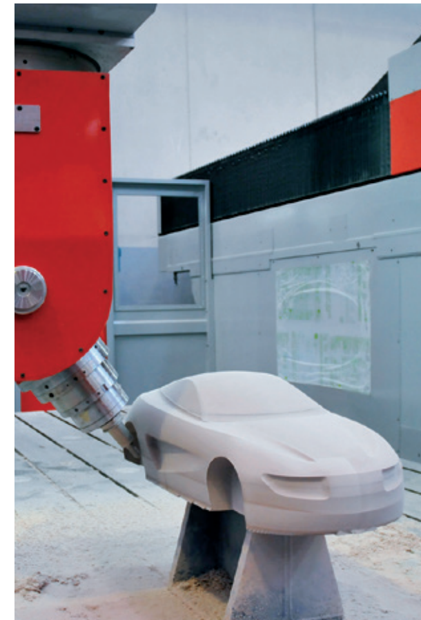
5-axis machining of a car model section for styling center
