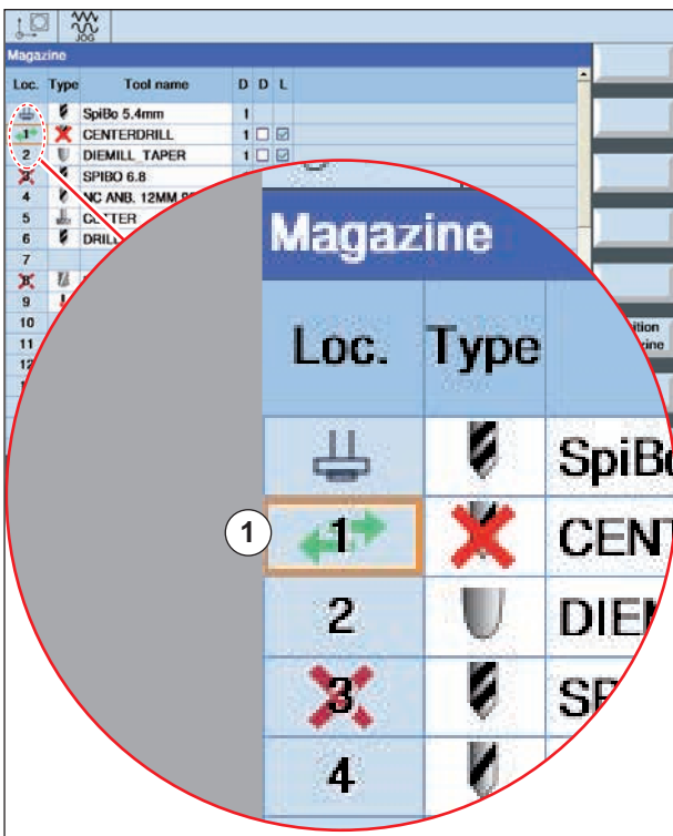
Magazine place is currently on the tool change point
