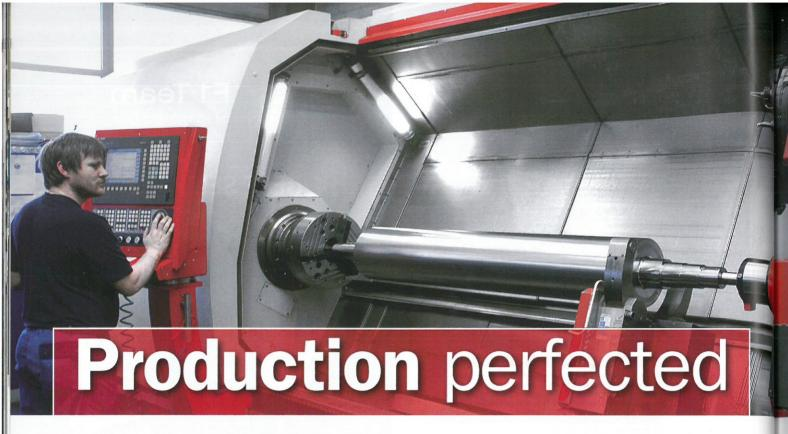
German firm Suchanke GmbH is a specialist in the manufacture of printing and embossing rollers made from materials such as St52, C45 and 42CrMo4, as well as Hastelloy 4893 and 4856. Emco Group turning technology supports its activities
