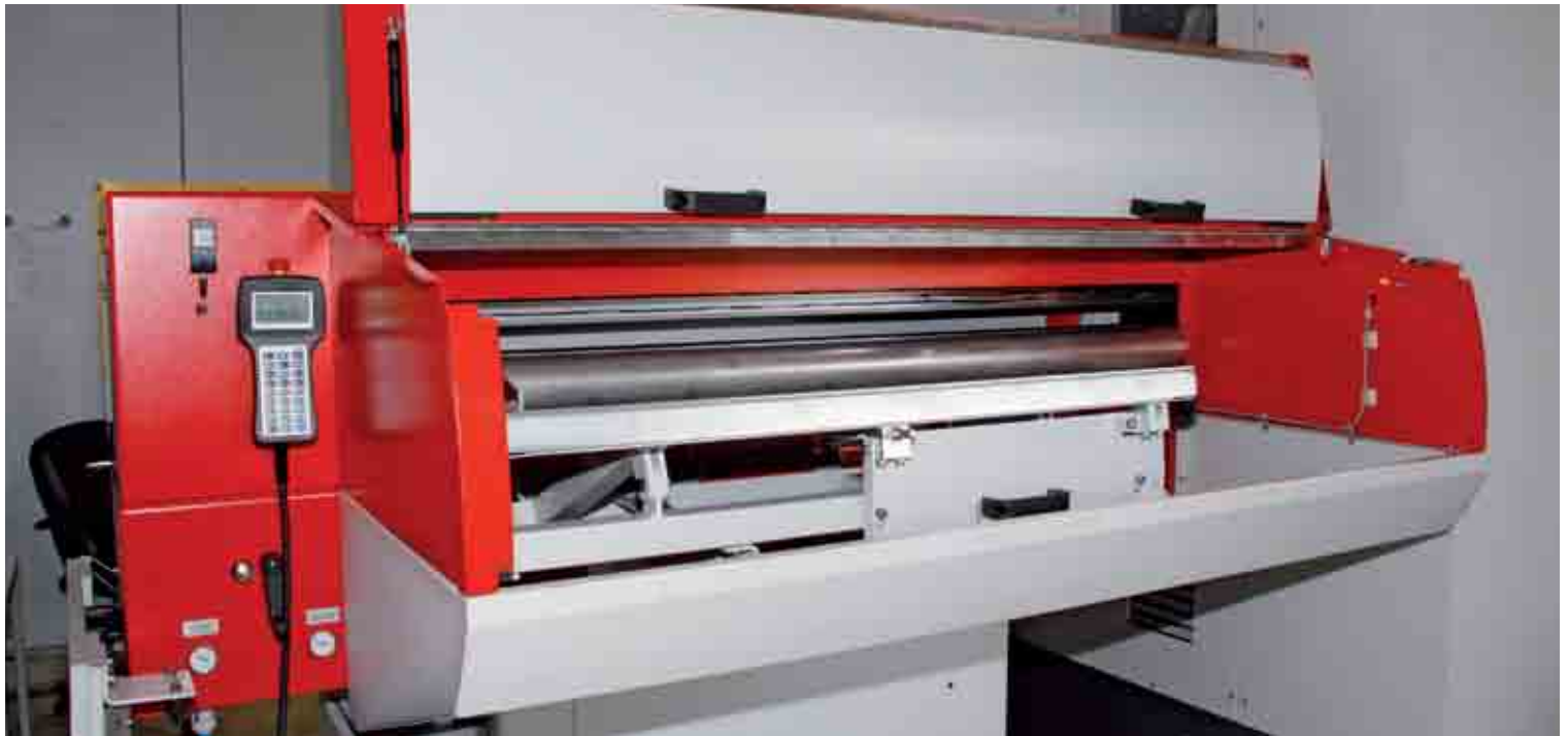
MKE's newly developed LM 1500 F bar-feeder provides for ergonomically efficient loading of bars up to Ø 95 mm at a small footprint.
