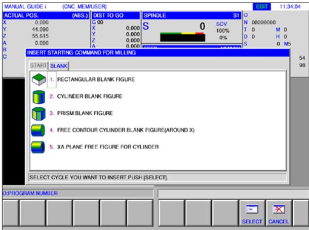
2 Select the register card for an unmachined part.
