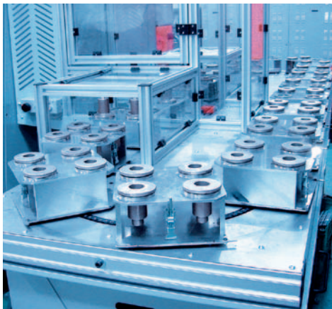
4-station pallet attachment for valve caps
