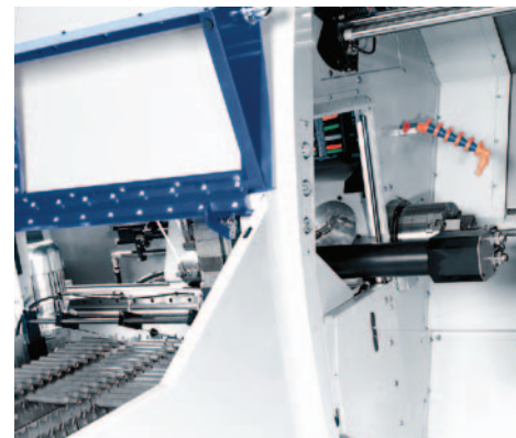
Fully automatic shaft loading. Feed-in via a conveyor belt, removal via the finished parts pick-up device.
