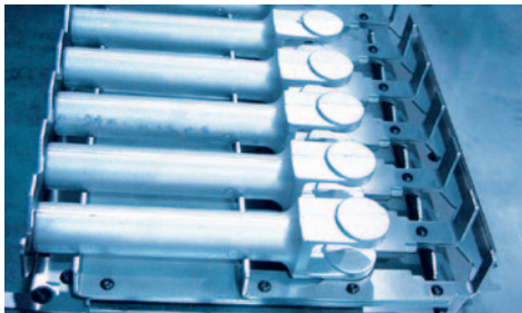
6-station pallet attachment for articulated brackets
