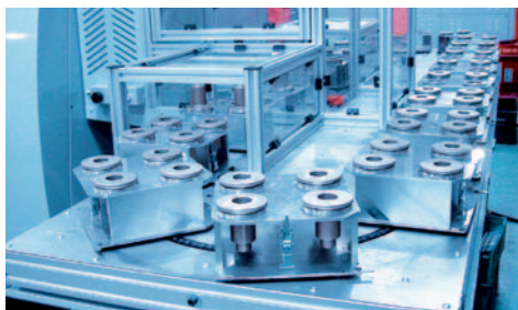
4-station pallet attachment for valve caps
