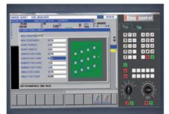
The change to a different control system is carried out within a minute by calling up the respective software
