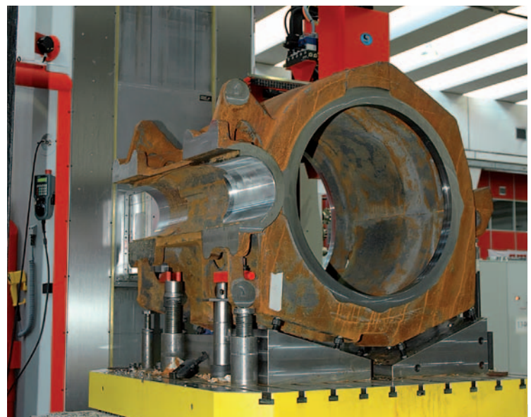
General engineering Machining a housing for an electric motor
