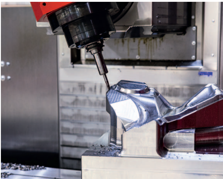
Simultaneous 5-axis machining with 45° B-axis (MMV 3200)
