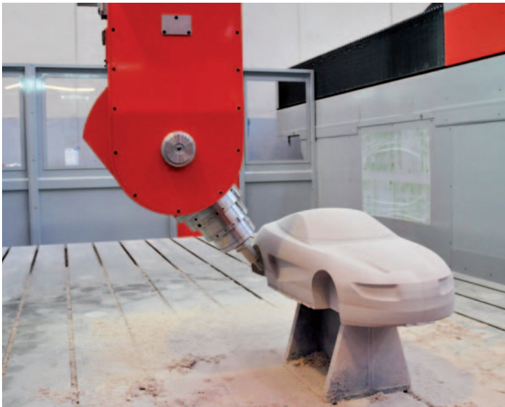
Automotive sector Machining of a scale model in resin
