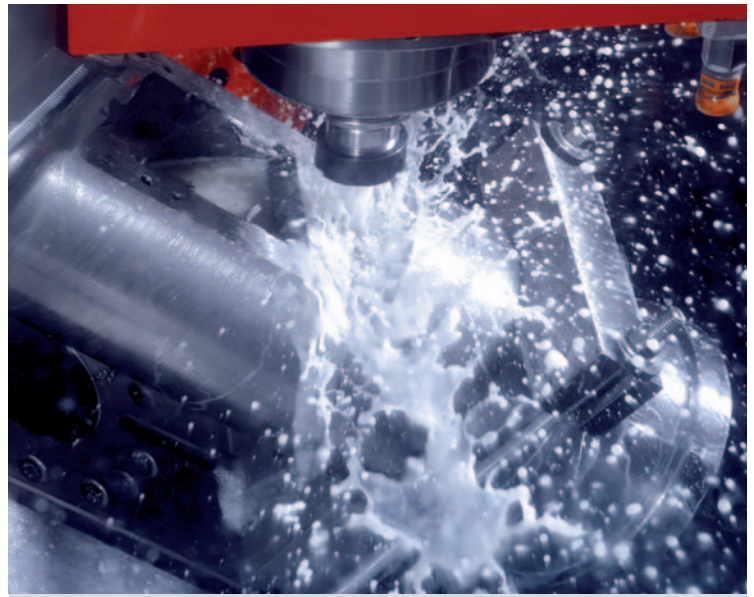
5-sided machining with rotary/tilting table (MAXXMILL 630-750)
