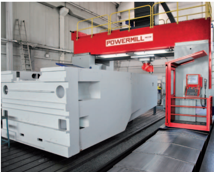
General engineering Machining of a large-dimensioned column for a machine tool
