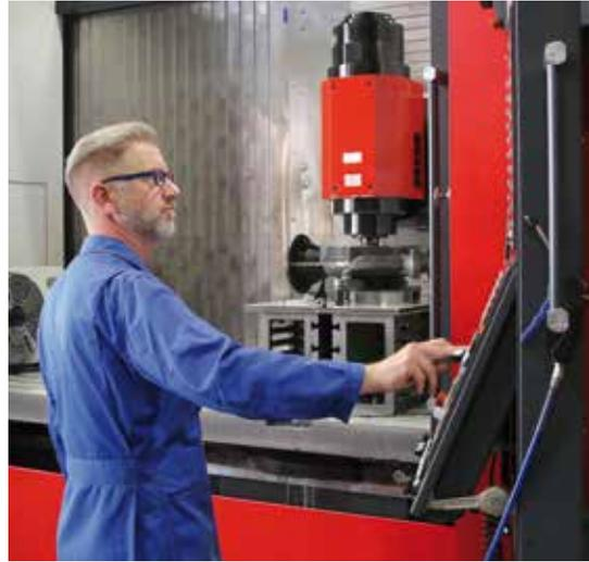
Thanks to the clever installation and use of space, efficient multi-machine operation can be performed by just one person. Because the design and spindle performance are identical, components can also be swapped between the machines quickly and flexibly.
