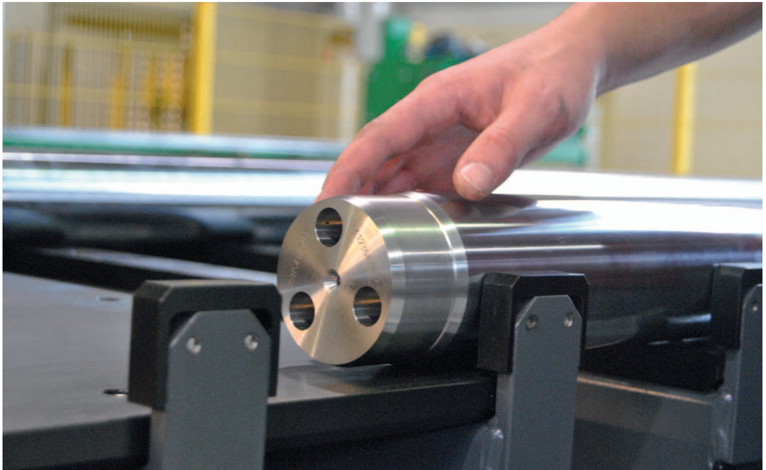
Among Stahl Judenburg's successful specialties are chromium-plated, stainless steel piston rods for hydraulic applications. Amongst other things, these have to be marked on the face side.
