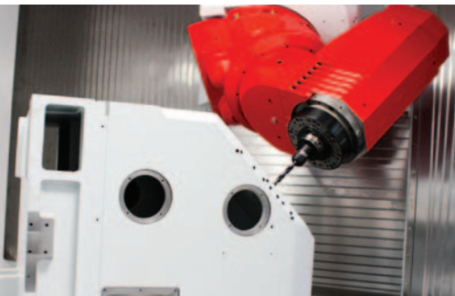
Milling, drilling and tapping on a milling head holder saddle
