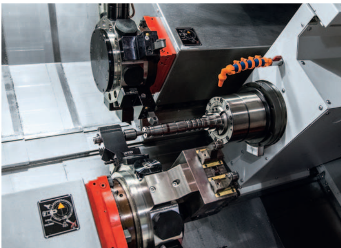
Live-center / turret-steady-rest. For complete machining of shaft work on the one hand in the main spindle and on the other hand in the sub-spindle, there are a live center and if needed also a turret steady rest available. So that long, slim workpieces can be manufactured precisely and without chatter marks.
