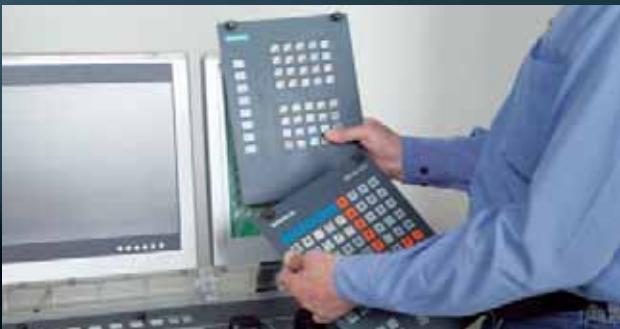
The unique concept of the interchangeable control can be fitted in all Concept machines. In doing so, the user is trained on all CNC industry control units that are common on the market.
