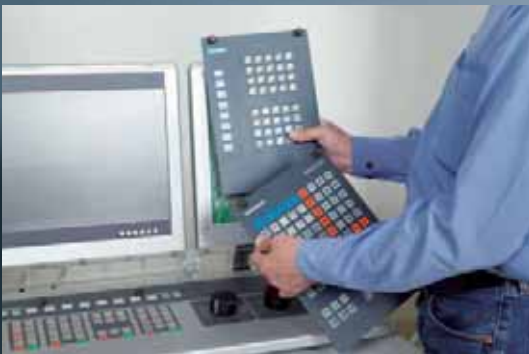
The conversion to another control system is carried out within a minute by calling up the respective software and by simply replacing the controller specific module.
