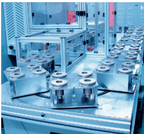
4-station pallet attachment for valve caps
