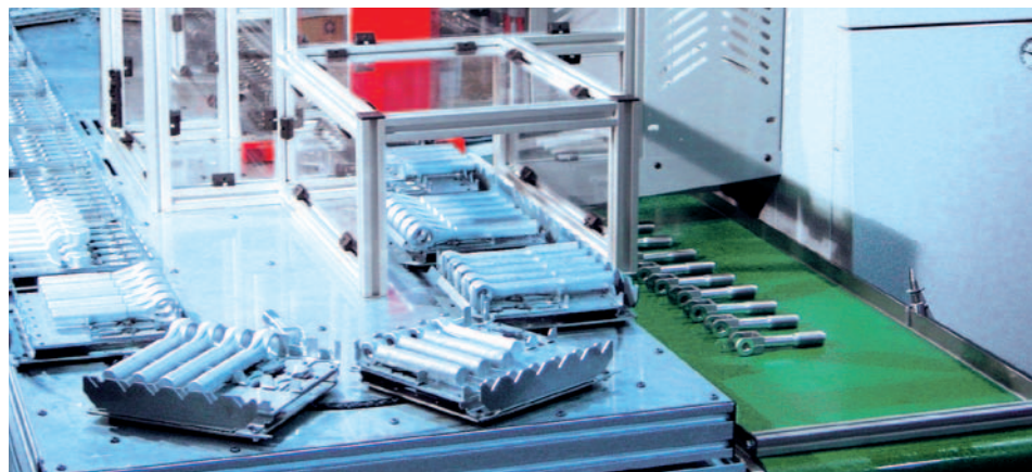
20-station pallet magazine with customer-specific pallets
