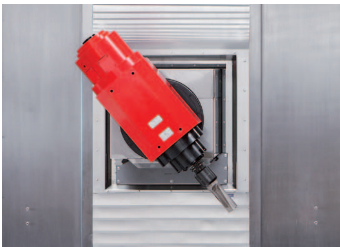
B-axis: The B-axis is driven by a torque motor, therefore achieving highly dynamic axis travel within the pivoting range of \pm 120 degrees.
