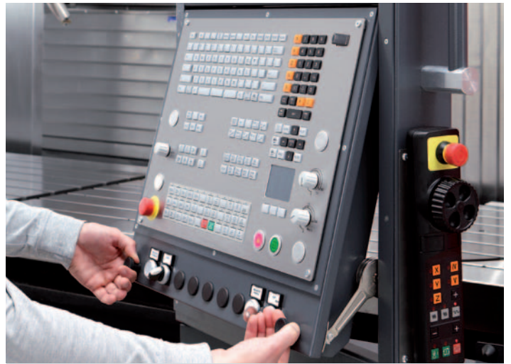
Control unit: The operator panel can travel, rotate and be adjusted in the direction of the work space. This ergonomic design provides ideal working conditions for the operator.
