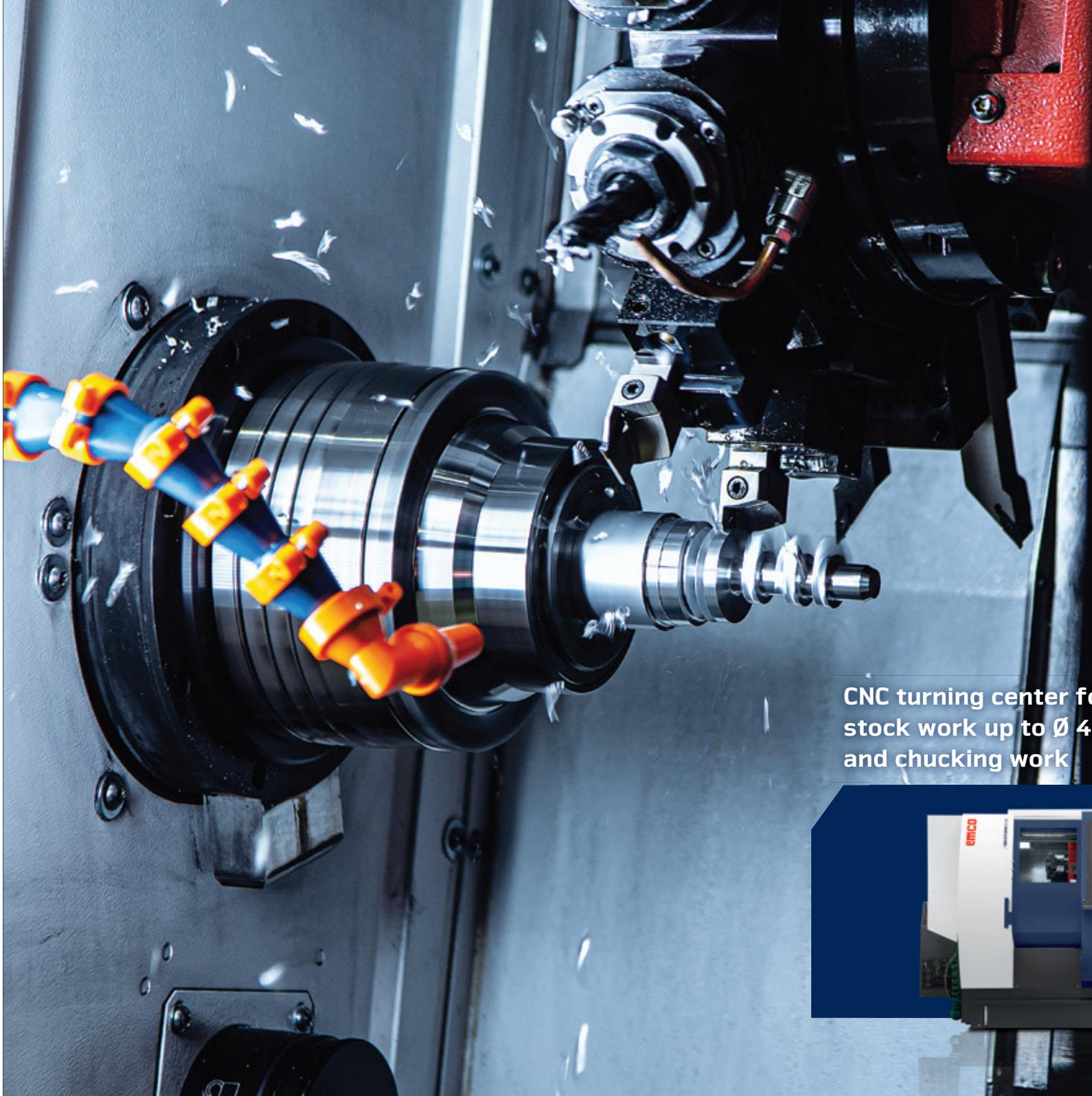
CNC turning center for bar stock work up to  $\varnothing$  45 (51) mm and chucking work
