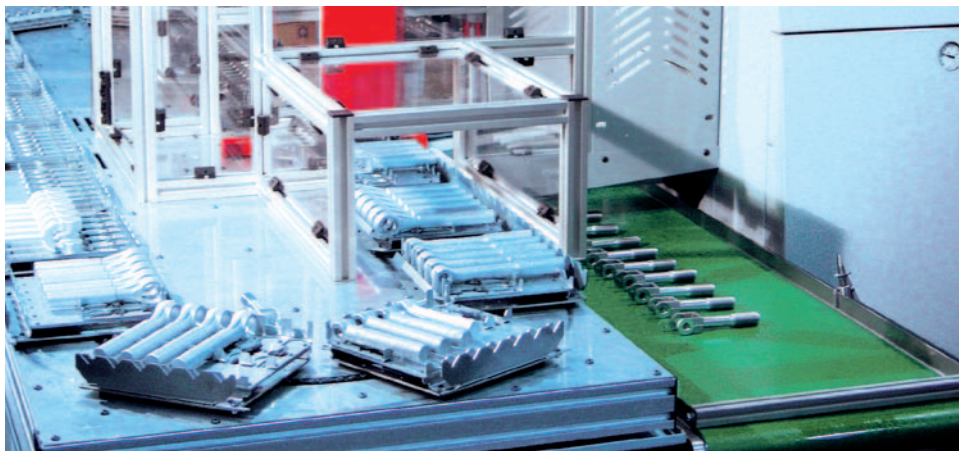
20-station pallet magazine with customer-specific pallets
