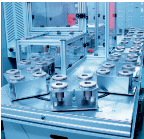
4-station pallet attachment for valve caps
