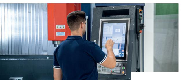
The EMCOMILL is equipped with state-of-the-art control technology, either Siemens 828D with ShopMill, Heidenhain TNC 620 or Fanuc Oi-MF with Manual Guide i are available. The control panel includes a swivel function for an ergonomic working position.
