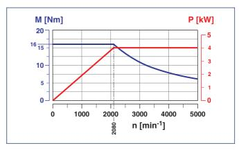
Motor characteristics for axial tool turret VDI 30
