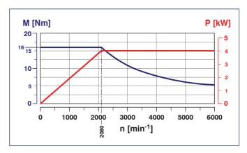
Motor characteristics for radial tool turret VDI 25
