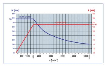
Motor characteristics for main spindle
