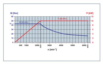
Motor charasteristics for counter spindle
