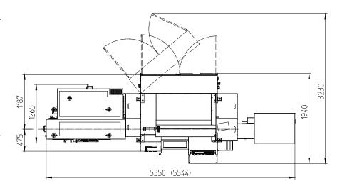
Machine layout E45 with EMCO SL 1200
