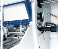
Shaft gripper for automatically loading pre-formed shafts.
