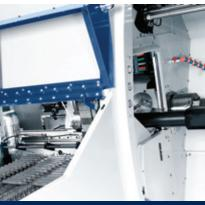
ully automatic shaft loading. Feed-in via a conveyor belt, emoval via the finished parts pick-up device.
