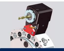
The angled workpiece holders provided by EMCO are delivered along with a precise alignment plate. Thus, it is not required to align the holders in the machine. The parallelism of the locating bore to the main spindle axis is guaranteed by the precise adjustment plate attached to the holders.
