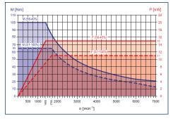
HYPERTURN 50 main spindle / counter spindle
