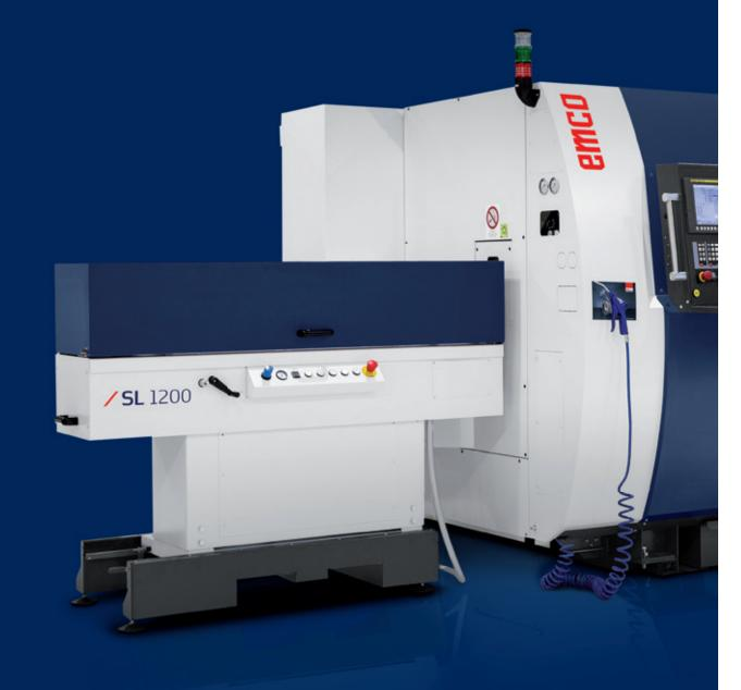
The EMCO SL 1200 is the perfect solution for automatic feeding and loading of cut-to-length bars. The key advantages are a small footprint and rapid loading times resulting from shorter strokes.
