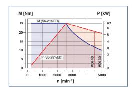
Milling drives in tool turret with VDI 30/40
