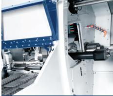
ully automatic shaft loading. Feed-in via a conveyor belt, emoval via the finished parts pick-up device.
