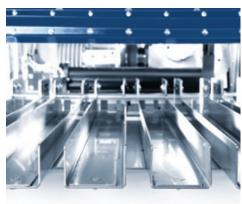
Multiple infeed chutes for loading rotationally-symmetrical blanks. The length of the blanks determines the number of
