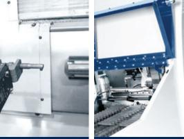
Shaft gripper for automatically loading pre-formed shafts. anks. A sensor monitors the availability of blank parts for each
