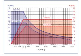
Main spindle / counter spindle motor characteristics
