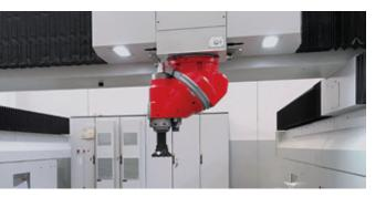
Z-axis saddle integrated in the machine crossbeam, its structure ensures highest stiffness results and utmost dynamic.
