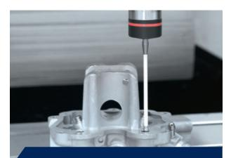
Tools measurements to reduce setup times during tool changes, as well as workpiece measurements to verify dimensions or to find zero locations. The optional workpiece measurement has a radio transmission, the tool set-up will be done by laser.
