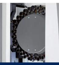
Drum configuration with dual arm grippers for fast tool chan-ges. Random tool management reduces tool changing times to a minimum. Thanks to the lateral magazine door (2x in case of double tool magazine), it is possible to check and set up the tools in parallel with the machining process.
