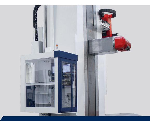
POMO and POVT Operator paltform with vertical (up to 2500 mm) and cross travel (up to 800 mm).
