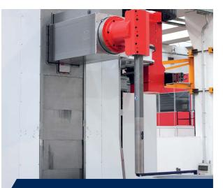
Turning head for supporting a special boring bar: 120 mm diameter, length up to 1500 mm for turning operations up to 1000 mm depth.
