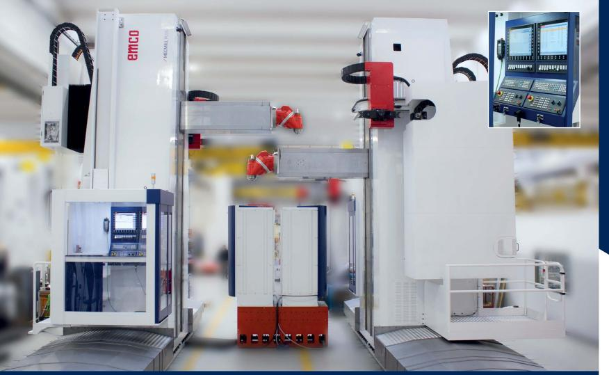
Opposite machines - Master and slave machine with master and slave CNC. The milling center is equipped with SANT-anticollision software.
