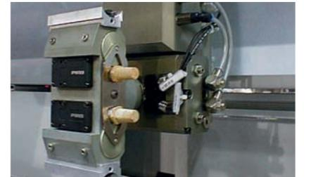
Vacuum suction gripper for fragile blanks
