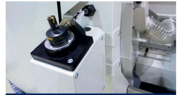
Balluff's "Easy Tool-ID" tool identification system makes it possible to start with automated tool management
