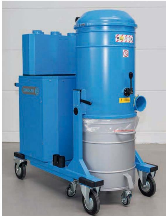
Stationary extraction unit for removing the plastic chips
