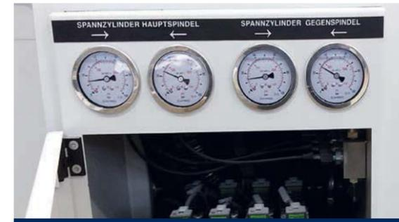
Thanks to the **differential pressure regulation** it is possible to fine-tune the clamping pressure for thin-walled workpieces
