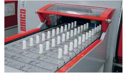
Blank feeding with indexing conveyor
