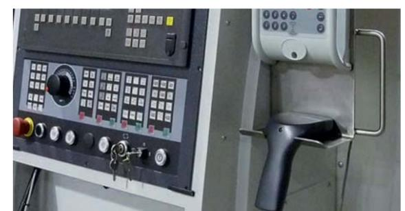
Using the barcode reader it is possible to scan and process job data
