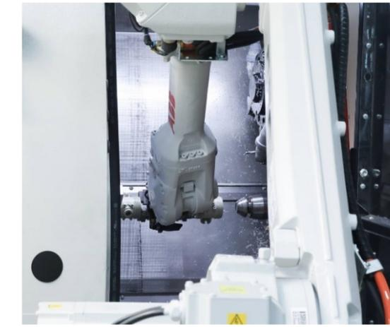
By means of a double gripper system, the plastic parts to be processed are safely transferred to the collets with a reduced clamping force.
