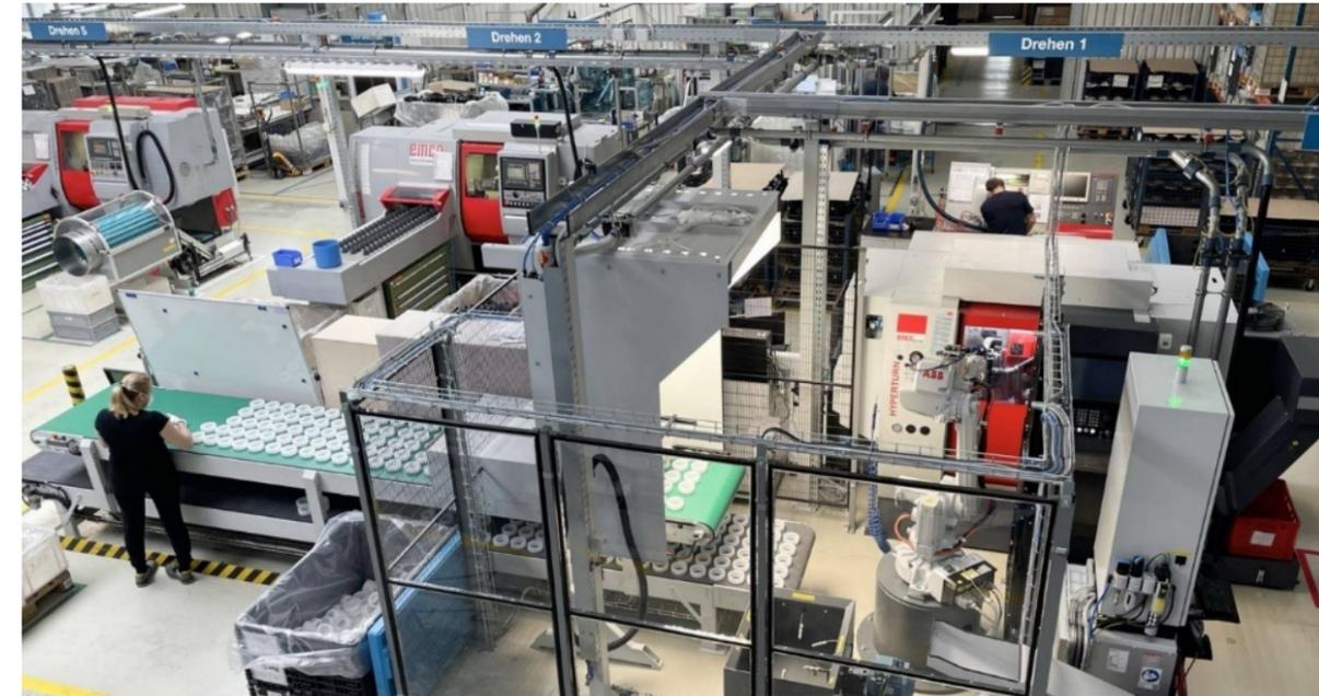
Praher's automation cell consists of an Emco Hyperturn 45 turning and milling centre, including chip extraction, and an ABB Flexloader™ FP600 robot cell with deburring station and blowing unit.
