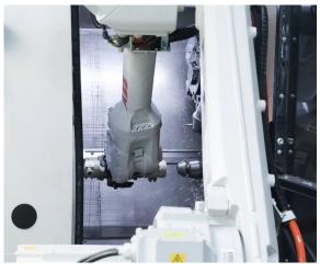
By means of a double gripper system, the plastic parts to be processed are safely transferred to the collets with a reduced clamping force.
