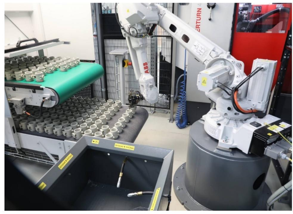
Praher produces around 5,000 different variants per year in typical batch sizes of 1,000 to 5,000 pieces. The MI DN25 ball housing is completely reworked in the Hyperturn 45 in a single clamping operation.
