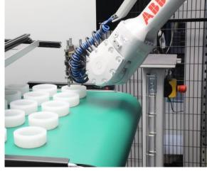
ABB's FlexLoader™ Vision system determines the position of the components. The coordinates are sent to the robot – the components can then be safely picked up from the conveyor belt and returned to the floor.
