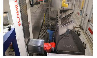
The Emco travelling column machine is used to machine H8 fits for shovels and arms as well as front and rear frames.
