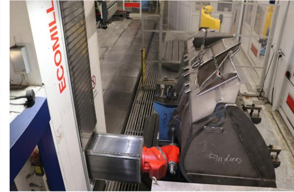
The Emco travelling column machine is used to machine H8 fits for different main components of Komatsu construction vehicles - shovels and arms as well as front and rear frames.
