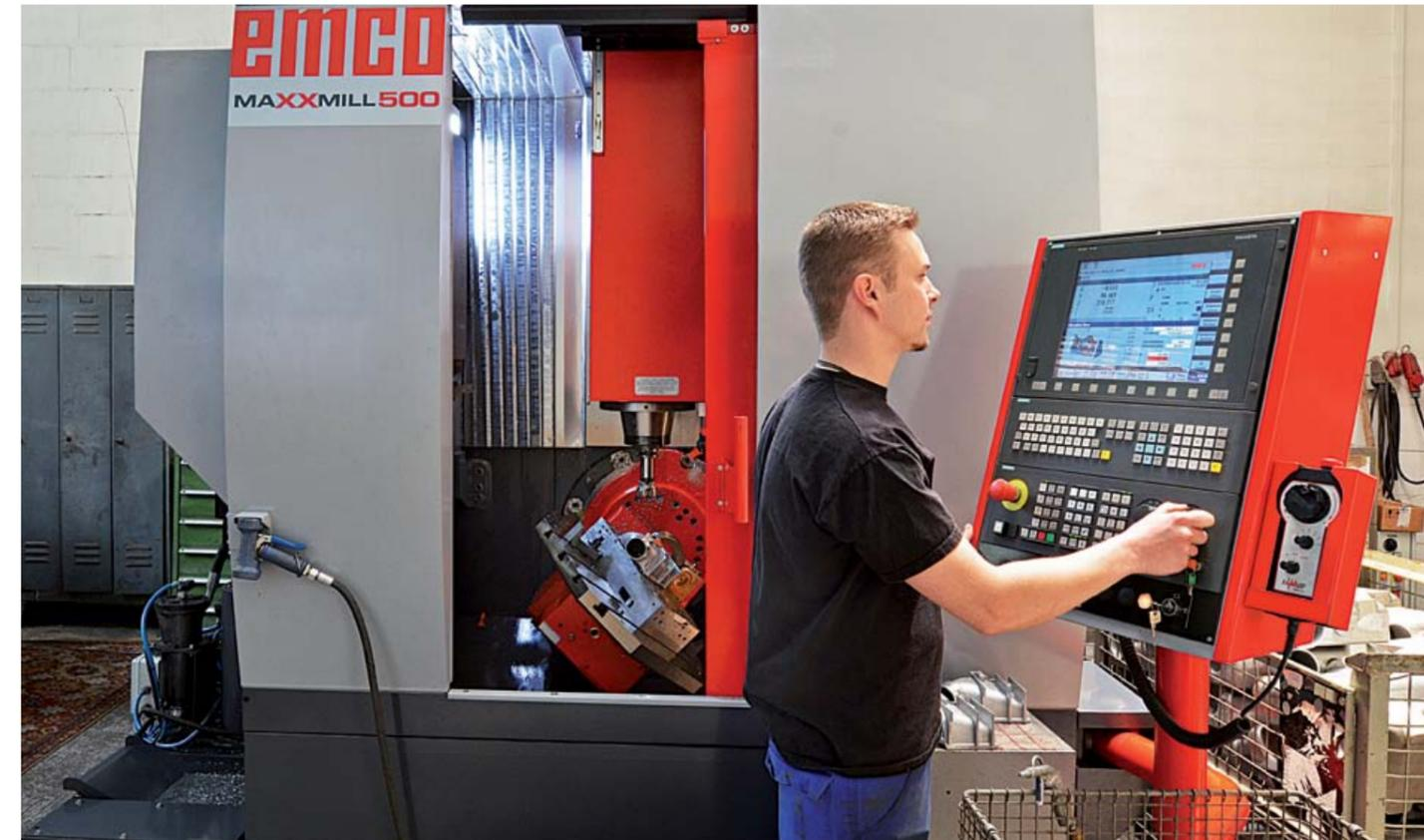
Maxxmill 500: vertical machining center for 5-axis machining
