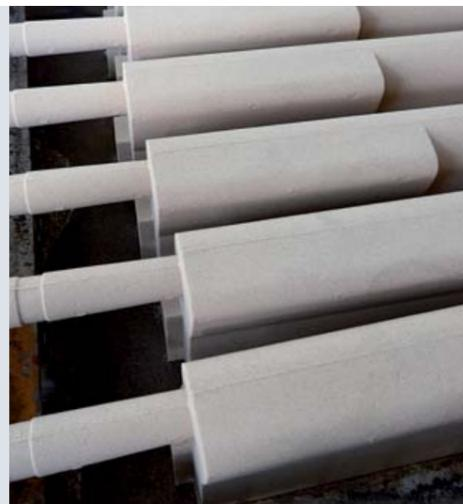
Compressed sand casting cores
