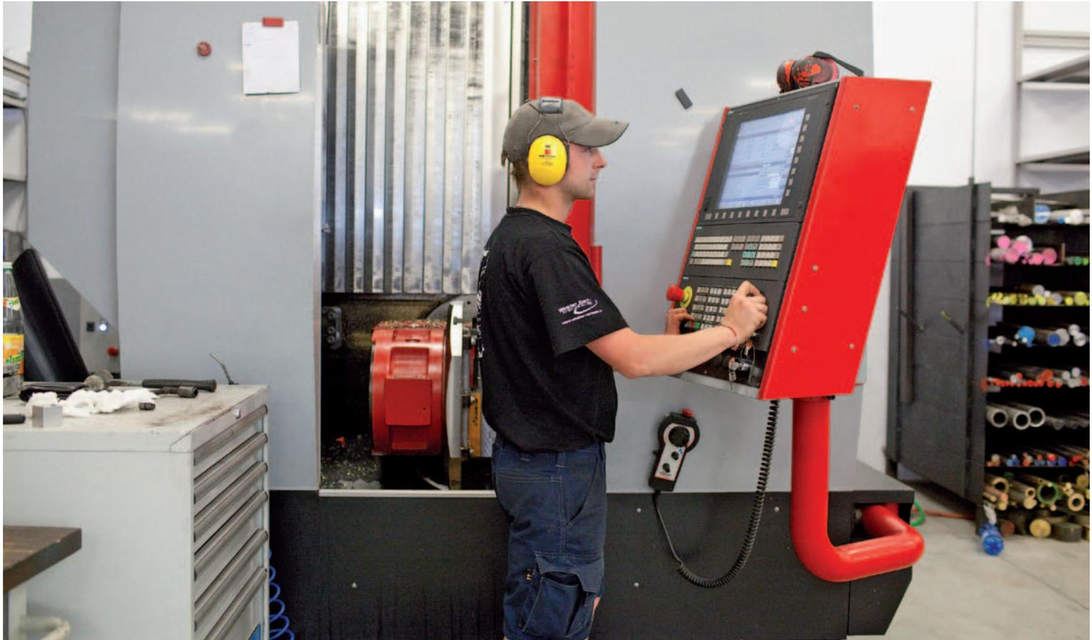
Complete production in a single clamping cycle. The specialists at Weico Mechanical and Metal Engineering have seen how the MAXXMILL 500 has met and exceeded this expectation. A shorter production time and machining in a single clamping cycle result in greater efficiency and precision.
